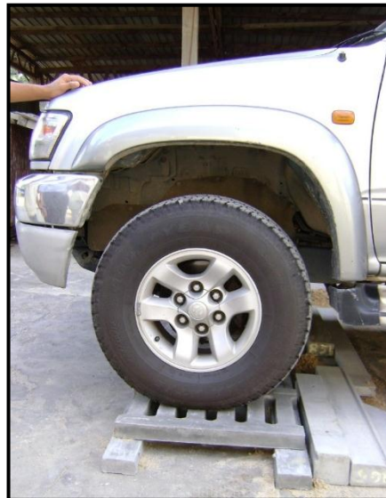
CONCRETE DRAIN COVER (600 X 390 X 50thk) CSL-CDC001
